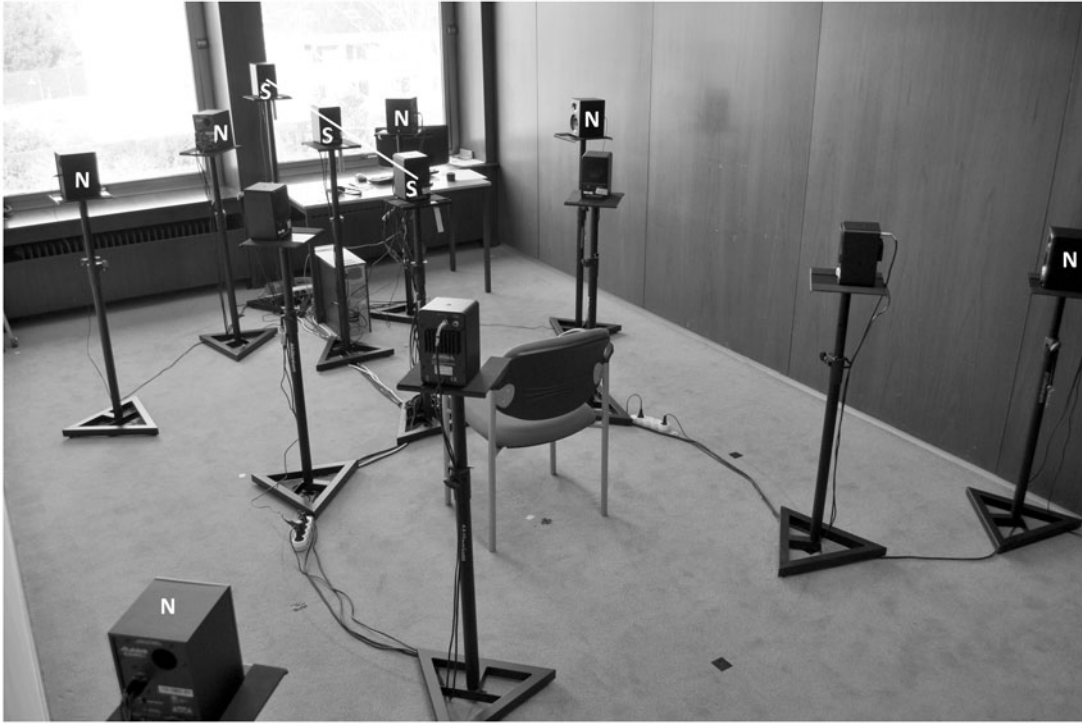
Figure 2. The test set-up of the room showing speaker locations. The CI user is seated at 1 m from the first speech speaker. The other two speech speakers are at 2 and 3 m in front of the CI user. Six noise speakers are positioned in the room to assure a uniform multitalker babble noise field. N: Noise presenting speakers; S: Speech presenting speakers.
