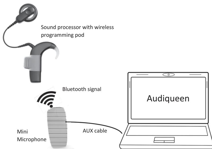
**Figure 1** Schematic drawing of the Coala Link setup.
